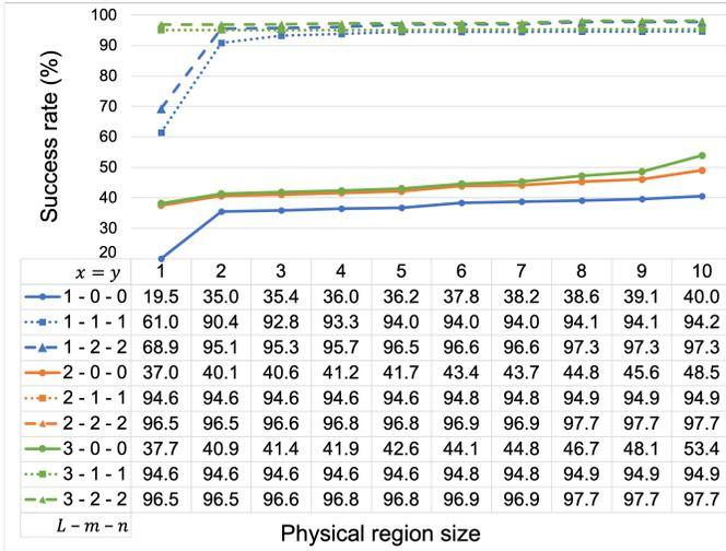
Fig. 3: Faulty function extraction success as a function of PEPR parameters  $x$ ,  $y$ ,  $L$ ,  $m$  and  $n$ .
