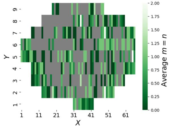
Fig. 4: Wafer map detailing average added logic levels  $m = n$  required for faulty function identification. (Gray locations did not provide any failures for analysis.)
